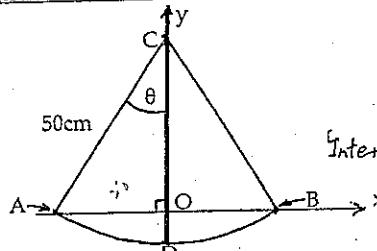
CA is a pendulum of length 50 cm oscillating uniformly about the vertical position, CD, so that the end of the pendulum describes the arc ADB and return in 4 seconds.
