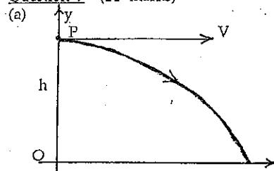
A particle is projected horizontally from a point  $P$ ,  $h$  metres above  $O$ , with a velocity of  $V$  metres/second. The equations of motion of the particle are
